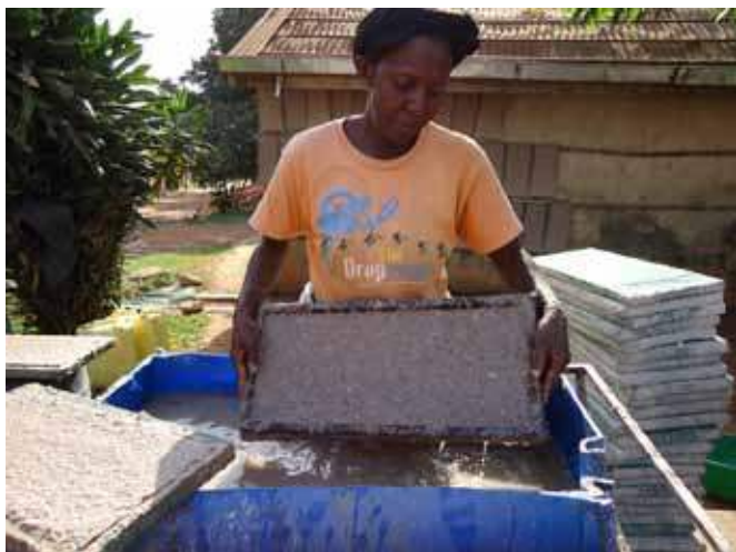
Making MakaPads, Makere University, Uganda (Photo: MakaPads Project, Technology for Tomorrow Ltd)
